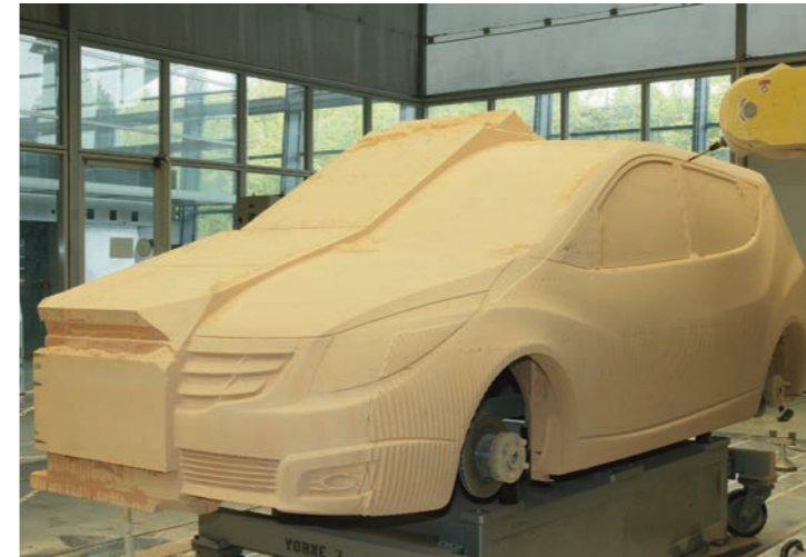
Full scale car model made of SikaBlock® M330 boards bonded with SikaBiresin® B260
