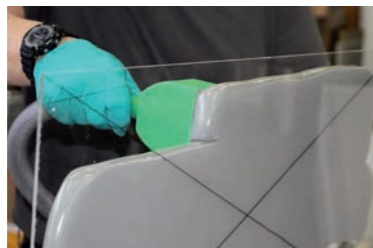
SikaBiresin® SC175 thixotropy enables vertical application in single layer and without sagging
