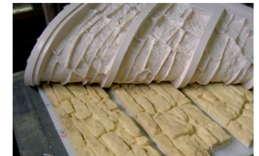
Release of SikaBiresin® UR548 soft mould for stone facing
