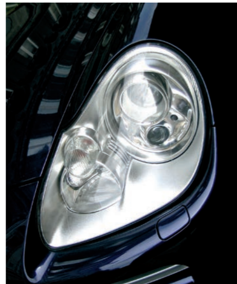
Front light lens made of SikaBiresin® PX521 / PX522
