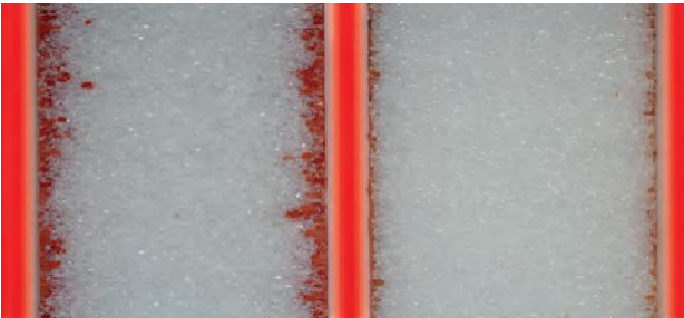
Photo of infused PET core materials with red-colored resin and removed skins. Commercially available PET foam 100 kg (left) vs. AIREX T92 SealX (right).
