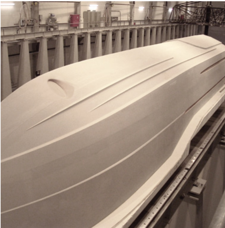
43 m long boat hull made of SikaBiresin® SC175 with a perfectly smooth and seamless surface
