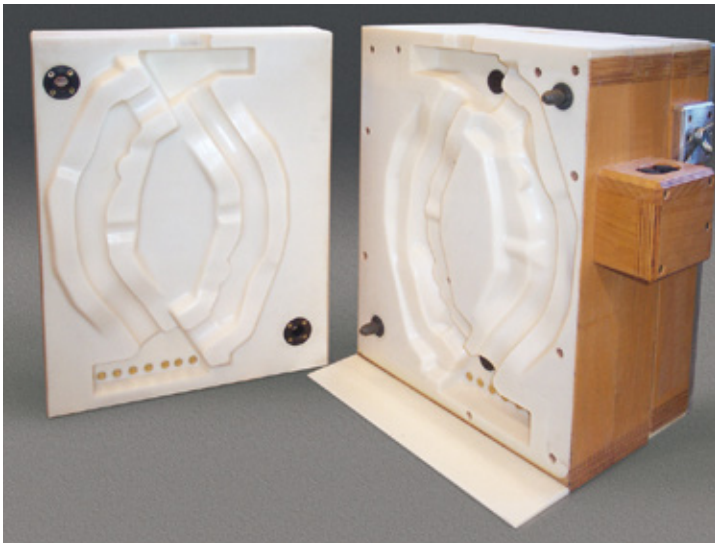
Core box made of SikaBiresin® UR132
