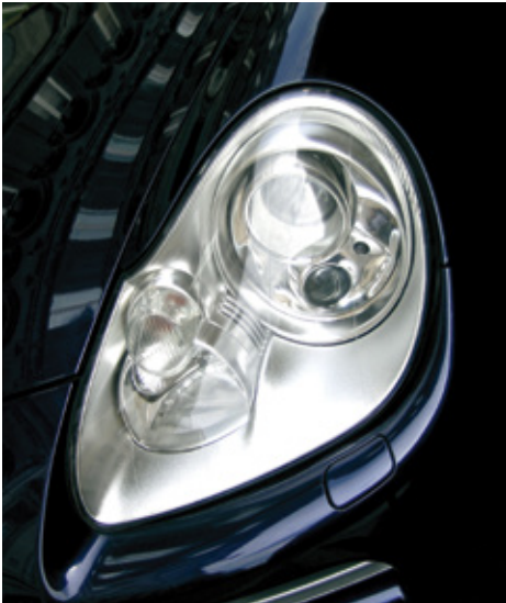
Front light lens made of SikaBiresin® PX521 / PX522
