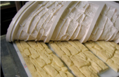
Release of SikaBiresin® UR548 soft mould for stone facing
