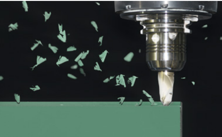
SikaBlock® M945 provides excellent milling behavior with low dust formation
